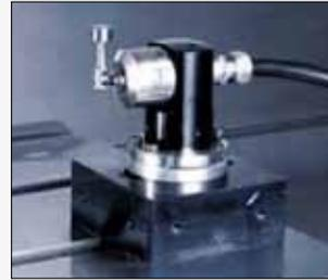
Automatic tool length measurement device
